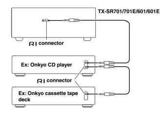
To connect components using the RI terminal, simply connect a remote control cable from this RI terminal to the RI terminal of the other component. An RI remote control cable with a 1/8-inch (3.5-mm) miniature two-conductor plug comes with every cassette tape deck, compact disc player, MD recorder, and DVD player that has an RI terminal.
